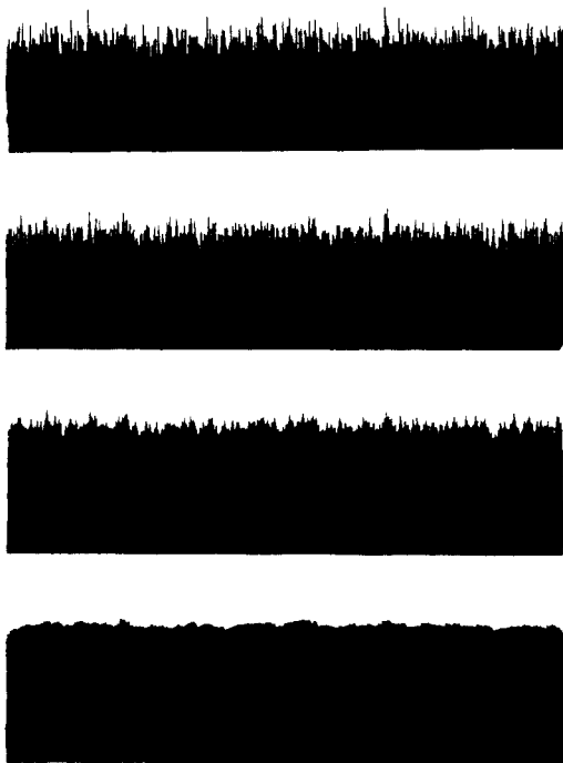
Figure 1. Typical deposits obtained for the threshold \Delta h = 0, 5, 10 and \infty . These simulations were performed with L = 600 and the maximum height 150. With decreasing \Delta h , the surface becomes smoother.
